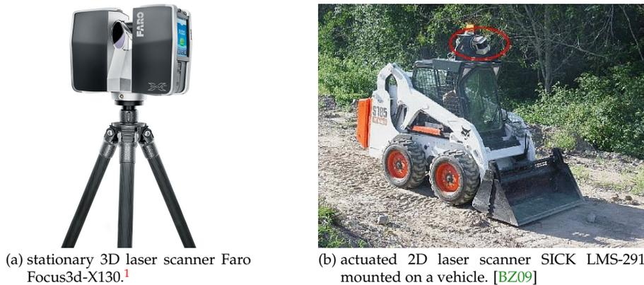
(a) stationary 3D laser scanner Faro Focus3d-X130.<sup>1</sup>
