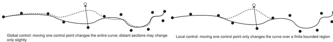
Figure 2.8: Global vs. local control [Par12, Fig 3.3]
